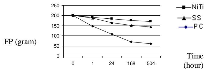
Figure (3): Force – time diagram of PC, NiTi CCS and SS CCS in mouthwash solution.
