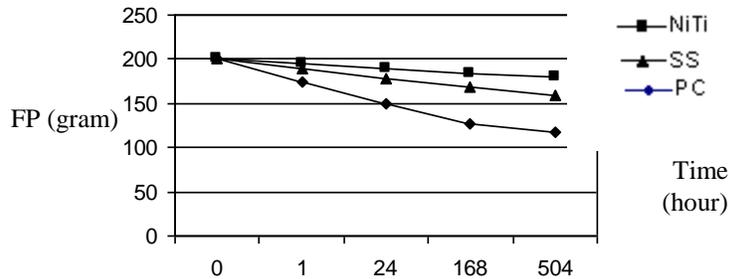
Figure (1): Force – time diagram of PC, NiTi CCS and SS CCS in dry condition.
