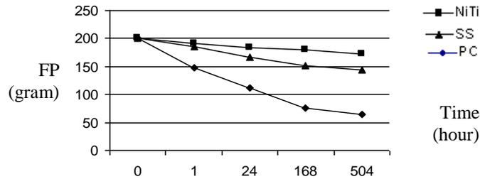
Figure (2): Force – time diagram of PC, NiTi CCS and SS CCS in artificial saliva of normal pH.
